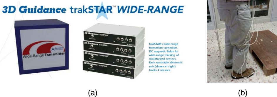
Figure 7. trakSTAR WIDE-RANGE measuring equipment with DC magnetic field transmitter [11] (a); remote sensor during measuring experiment (b)
