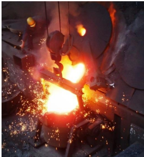
Figure 1. Pouring liquid iron from the furnace to transport pot
